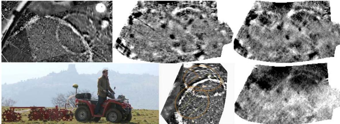
Figure 4. Magnetic map where is clearly visible one big circular feature, ERT maps at 50 cm, 1 m, 1.5 m dept where are clearly visible two big circular features, 3D visualization and draping of the magnetic map on the DGPS DTM with overlaid the ERT interpretation
