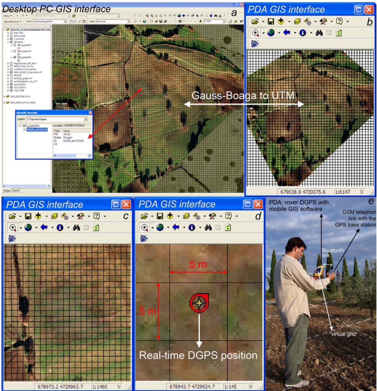
1-PDA mobile GIS at work: grid collection without the need to build a physical grid moving directly to surface collection
