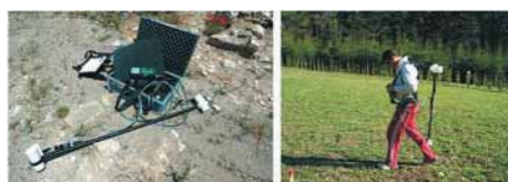
Fig. 2 - Magnetometro a protoni Overhauser.
